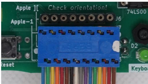
An Apple-1 keyboard connected with the pin-1 marking pointing to the right (J5 + J7).
