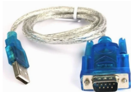
Cable example that needs an extra null modem cable
