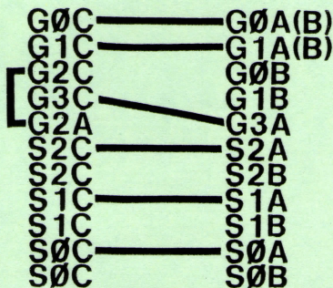
THIS CONFIGURATION WILL MAKE SOCKET "A" AN EXACT DUPLICATE OF THE GAME I/O SOCKET IN THE COMPUTER, ASSUMING THE SWITCH IS IN POSITION "A".
